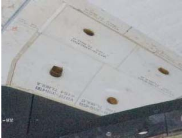
Figure 2. Protruding FRSI plug
